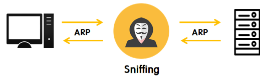
Fig. 1. ARP spoofing packet flow
